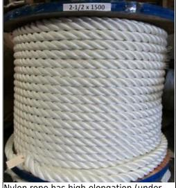
Nylon rope has high elongation (under load) when compared to other synthetic ropes. Nylon has high energy absorption under shock and good abrasion resistance. When combined, these characteristics makes nylon rope the best in handing compared to other synthetics. It's utilized extensively in marine use such as mooring lines, towing slings, commercial fishing, utility rope, leasure boat, sailing etc.
