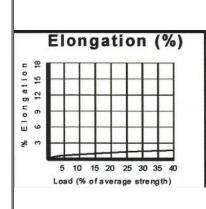
0.98\* Specific gravity Melting point 284° F (140° C)° 150° F (65° C)° Critical temp. 0.09-0.12\* Coefficient of friction Elongation at break 4%.5% Fiber water absorption 0% UV resistance moderate Wet abrasion superior Dry abrasion superior
