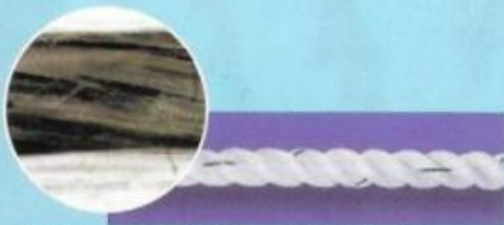
The fiber construction of general Polypropylene rope.
