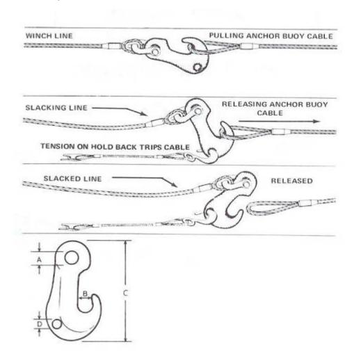
Marine Anchor Line or Cargo Hook Cast High Strength Alloy Steel
